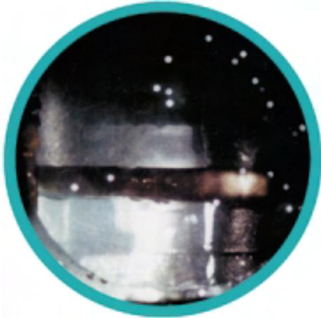
The compressor can therefore experience a loss of lubricant quality, washout of oil from the bearings, a sudden reduction of the amount of oil in the compressor, the potential for mechanical damage to the compressor due to liquid slugging as oil is carried through, as well as very high compressor discharge pressures which further add to the possibility of mechanical component failure.
