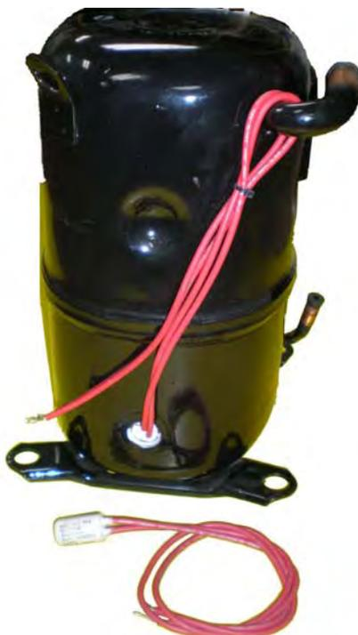
Because the shapes of the heater and the surface of the well will not match perfectly, and there needs to be clearance to allow easy assembly, heat transfer will be impeded unless a thermal paste is used when locating the heater in the well. This thermal paste fills the gaps, and assists in the transfer of heat from the CCH to the compressor.
