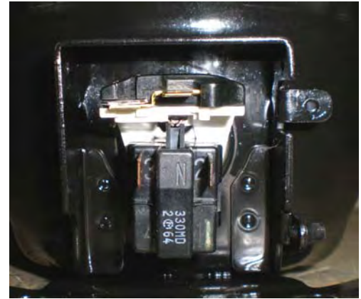
AZA refrigeration compressor with the thermal protector and relay assembled
