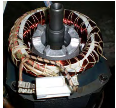
AW refrigeration compressor with the internal motor protector
